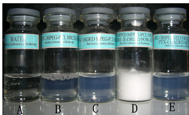
Fig. 4. Morphology of PTX-NPs. (A) Water, (B) Blank MPEG–PCL NPs (33 mg/ml), (C) PTX-NPs (DL=8%), (D) PTX-NPs freeze-dried powder, (E) Re-dispersed freeze-dried PTX-NPs with water (DL=8%).
